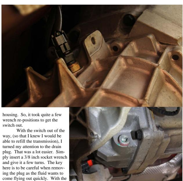
drain plug out, I pull out the jack
